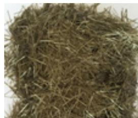
**Fig.2.** Chopped Basalt fiber
